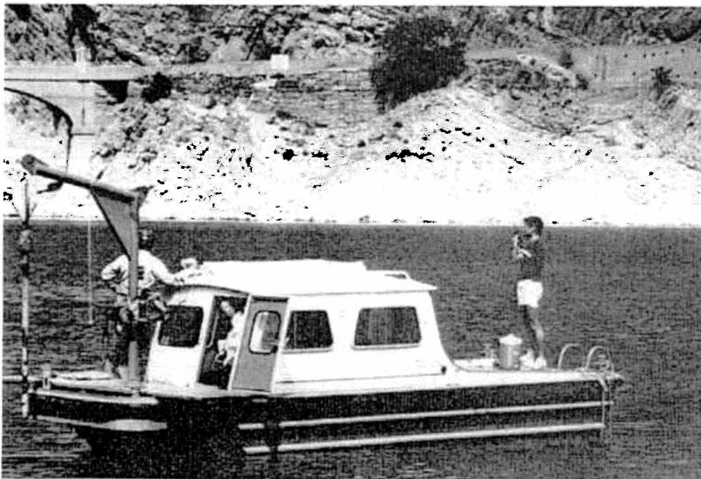
Figure 6.—Gravity core sampler mounted on boat for sampling operations. P801-D-80114
